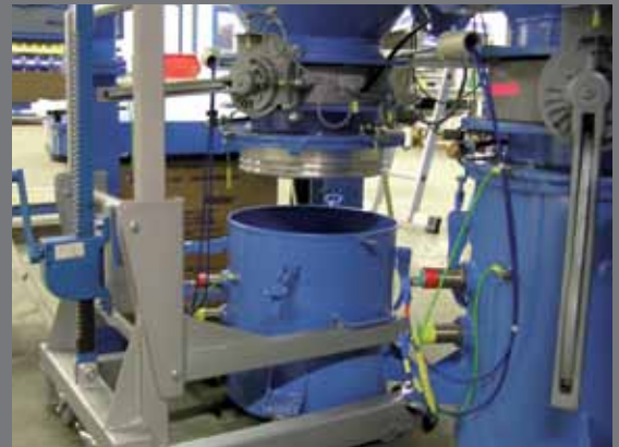
Lift cart for a safe dust bin change
