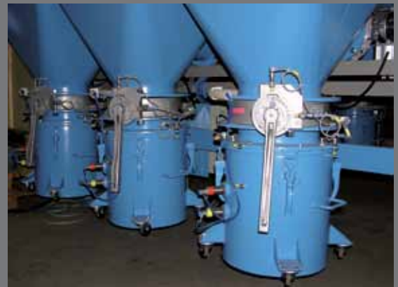
Dust collecting bin with contact sensors
