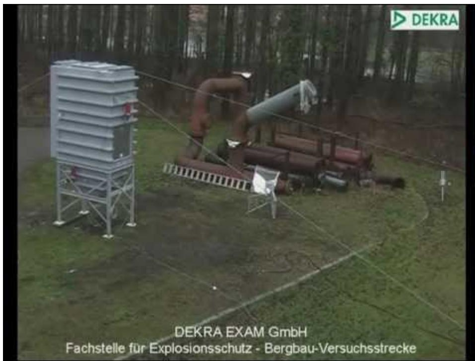
As proof of the pressure shock resistance, the DEKRA executed two explosion testings of a pocket filter type AJN 1/603 SL on ...
